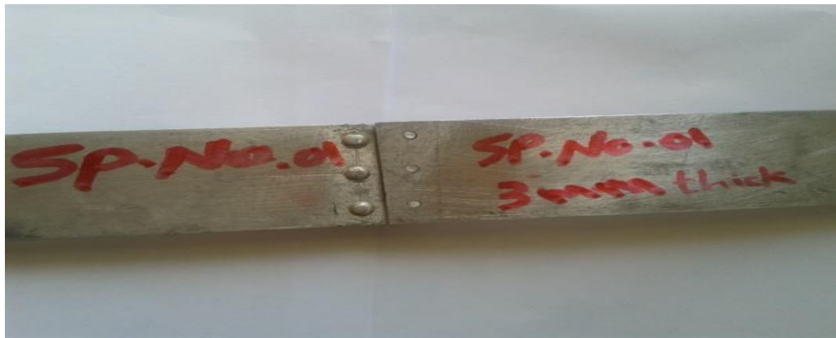
Figure (3): Specimen and rivets after tensile strength test
